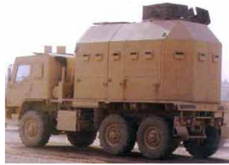
HUNTSVILLE, Ala. -- Teledyne Brown Engineering, Inc. has developed, built and tested an armored troop carrier system, the Multipurpose Troop Transport Carrier System (MTTCS), which is designed to protect soldiers from small arms fire and most fragments from Improvised Explosive Devices (IEDs).
