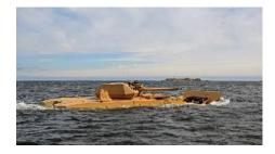
Patria AMV28A armoured wheeled vehicle completed successfully the swimming tests organised in the end of May in Finland. With a total weight of 28 tonnes the vehicle swam without difficulties, as expected. Patria AMV28A, where 28A stands for 28 tonnes GVW amphibious (sea-stage 3) vehicle, is the latest member of Patria AMV product family, introduced at IDEX 2017 event earlier this year.
