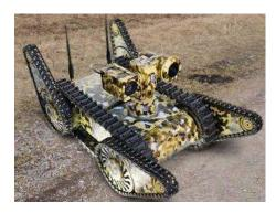
The newest engineering robot Kapitan has a modular layout and, depending on the tasks performed, can use various special equipment, which, thanks to a special docking station, can be installed within a few minutes. Among the tasks that can be performed using this platform are mine clearance, visual reconnaissance, in the future it is planned to deploy electronic warfare equipment on it.
