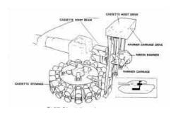
Autoloader (also called automatic loader) is a mechanical system to load the main armament and so eliminate one member (human loader) from the fighting vehicle's crew.
