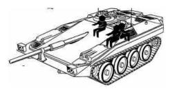
This is a turretless tank that features a gun fixed to its chassis rather than installed in a turret. This design offers a simple method of automatic loading and would permit a longer barrel to be used than would be possible in a turreted tank of similar size and weight.
