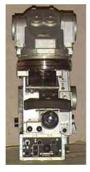
A sight based on the use of infra-red technology to produce a picture of the heat signature of an object against its background. It is a passive system which detects infra-red (IR) radiation emitted by the target and converts this into an electrical signal which can be used to create a visual image.
