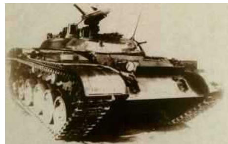
A tank destroyer, or a self-propelled anti-tank gun, is a type of armoured fighting vehicle. Tank destroyers are used primarily to provide antitank support in combat operations but do not fit all the criteria of a tank. They may mount a high-velocity anti-tank gun but have an open turret, no turret at all or run on wheels instead of tracks. Vehicles which carry a antitank guided missile launcher are referred to as ATGM carriers.
