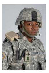
Designed for both mounted and dismounted infantry, QinetiQs miniature, low-profile acoustic Ears family of wearable, sniper detection and gunshot localisation solutions is based on a miniature single integrated acoustic sensor.
