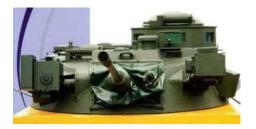
Denel Land Systems has expanded the day and night fighting capabilities of its LCT20 turret`s capabilities by integrating an advanced electro-optical sighting package for both the Commander and Gunner, this turret can be integrated into a wide range of armoured fighting vehicles.
