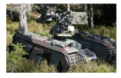
The Titan unmanned ground vehicle by robotic warfare systems developer Milrem Robotics with the PROTECTOR remote weapon station by Kongsberg Defence and Aerospace is exhibited at this year's AUSA trade show in Washington DC.
