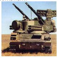
The Tunguska-M1 air defence system is fitted with both guns and missiles and is intended to protect armoured and mechanised infantry units against low-flying fixed-wing aircraft and helicopters, some types of cruise missiles as well as for defeating light armoured ground targets and personnel of the enemy.
