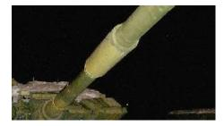
A bore evacuator (also called a fume extractor) is a device on the gun barrel of an armoured fighting vehicle which helps prevent poisonous propellant gases from venting back into the vehicle's fighting compartment when the gun breech is opened to load another round.
